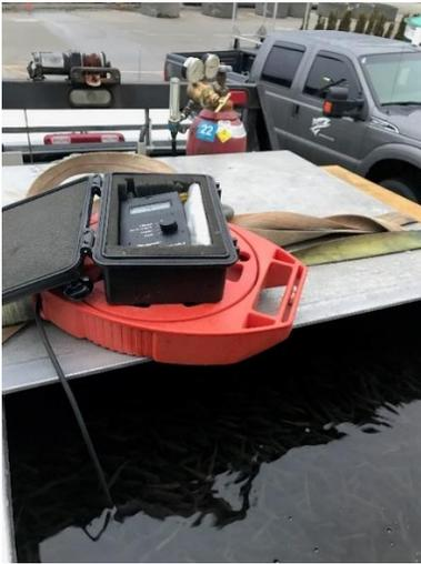
A dissolved oxygen meter is used to monitor the amount of oxygen in the water during loading and transport. It is important that oxygen levels don't increase or decrease to much as either can be detrimental to the health of the fish.
